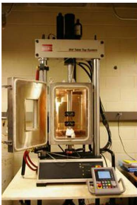
Fig. 5 Photograph of MTS 858 Hydraulic-Servo Test System
